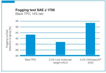
Heating in fog test chamber 6 hours at 110°C, chill plate at 38°C
