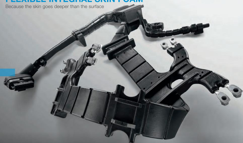
Although having an open-cell foam core structure, Elastofoam® I has been developed to form an integral skin as decorative and protecting surface in a one-shot process. Using water as a chemical blowing agent or physical blowing agents, Elastofoam® I reproduces the texture of the mold surface perfectly. Mostly in combination with an appropriate coating these flexible integral systems provide a soft, pleasant touch combined with a UV-, scratch- and abrasion resistant surface of smooth haptic.
