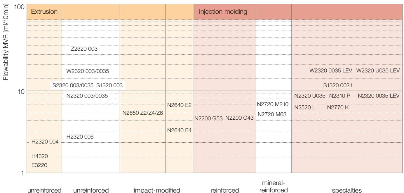
Fig. 19: Selection of grades from the Ultraform® range
