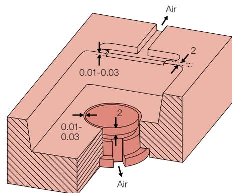
Fig. 24: Mold venting system
