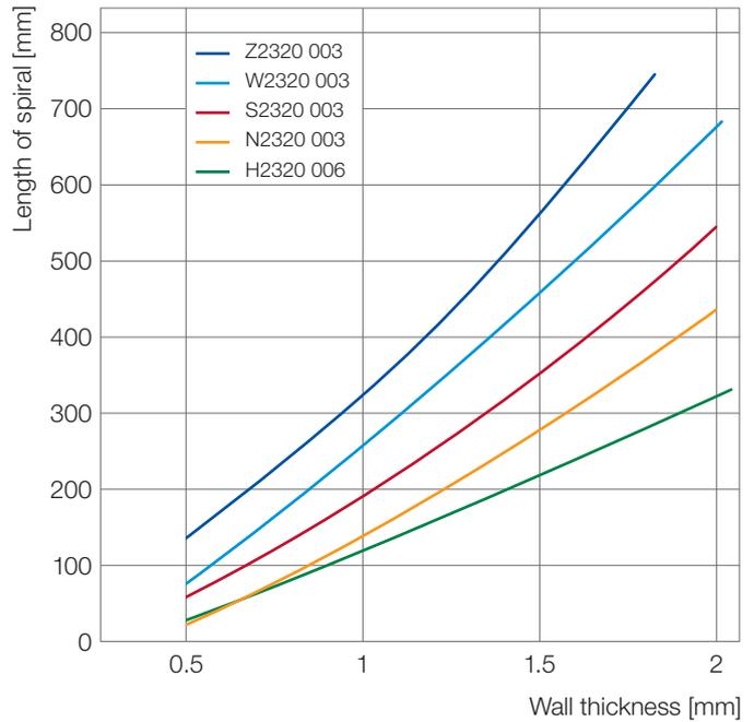
Fig. 25: Flowability as a function of wall thickness (spiral flow test). Machine: 1300 kN, screw diameter: 30 mm, mold: test spirals, injection pressure: 1200 bar, melt temperature: 210°C, mold surface temperature: 80°C
