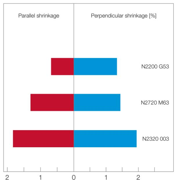
Fig. 31: Shrinkage of unreinforced, glass-fiber reinforced and mineral-filled Ultraform® parallel and perpendicular to the direction of flow for free shrinkage determined for sheet measuring 110·110·2 mm; melt temperature: 200°C, mold surface temperature: 80°C
