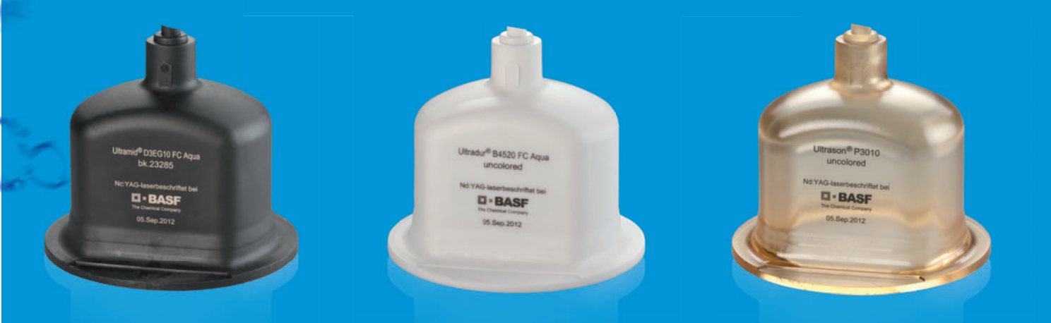
Fig. 3: Ultrasilim® Fatigue Testers made from Ultramid® D3EG10 FC Aqua (left), Ultradur® B4520 FC Aqua (middle), Ultrason® P3010 (right)
